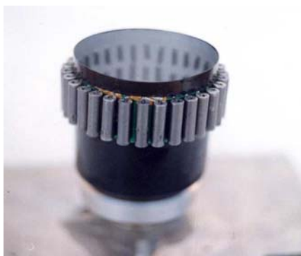
Fig. 9 Flexible rotor with ferromagnetic armatures mounted by means of the fixing anchors (practical achievement)
