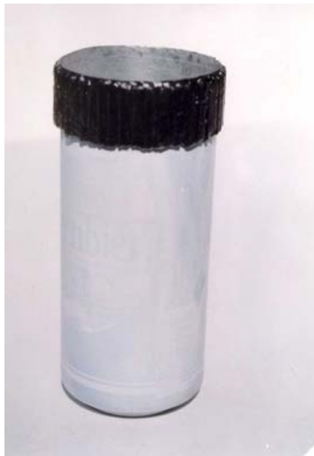
Fig. 4 Flexible rotor with ferromagnetic armatures of cylindrical bar, fixed with adhesive (practical achievement)
